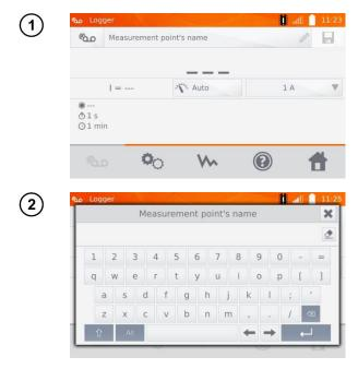
When necessary, name the measuring point.
