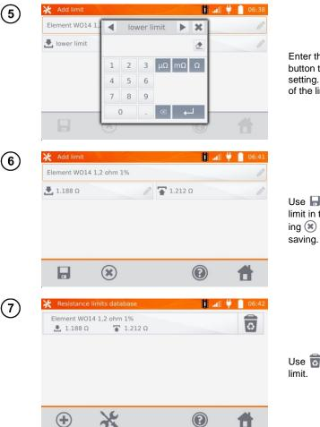
Enter the lower limit. Use button to go to the upper limit setting. You can set only one of the limits.
