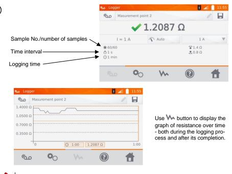
After the logging process, the result may be entered into the memory by pressing button (see sec. 4.2). The values of individual samples may be read by viewing memory (see sec. 4.3).
